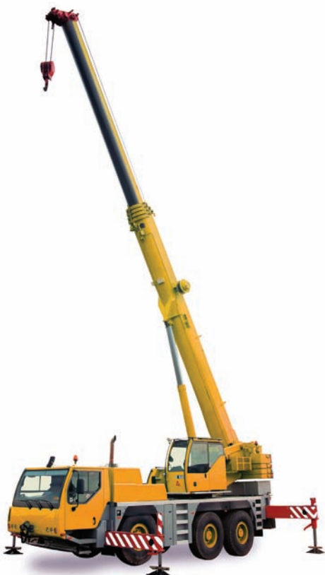
Application example for hydraulic cylinders in mobile use. As well as the support displacement, the extending movement of the stabiliser can also be measured
