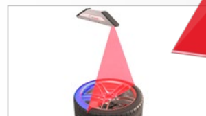
Inline 3D inspection of tire geometry
