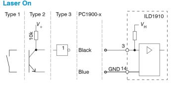
If pin 3 is not connected with pin 14, the laser is off.
