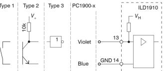
24 V logic (HTL): Low level  $\leq$  3 V; High level  $\geq$  8 V (max 30 V) 5 V logic (TTL): Low level  $\leq$  0.8 V; High level ≥ 2 V internal pull-up resistor, an open input is detected as High.
