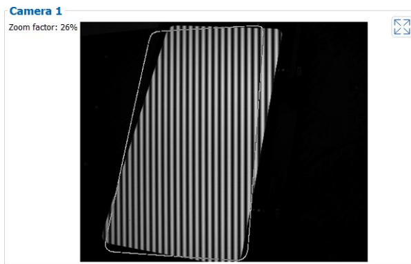
Fig. 3.6: Positioning the reference target – position has to be corrected
