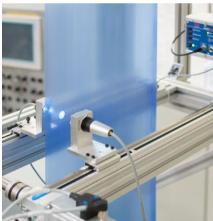
Inline measurement of the color gradient of glass, Plexiglas®, PET and PVC films and paper
